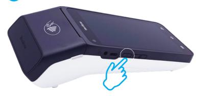
Press the power button on the side of the terminal.
