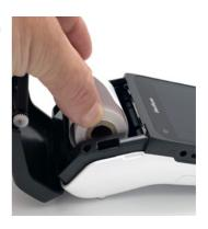
Remove used paper roll. Insert new roll so the paper feeds from the top, leaving a length of paper sticking out of the terminal
