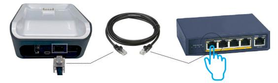
Plug one end of the Ethernet cable provided into the port labelled with the  $\frac{1}{100}$  icon on your T650p Full Feature base. Plug the other end of the Ethernet cable into a free LAN port on your router.
