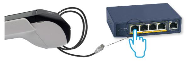
Plug the other end of the Ethernet cable into a free LAN port on your router. Look for the Ethernet icon **(•••)** at the top of the screen to confirm that your terminal is connected.
