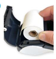
Remove used paper roll. Insert new roll so the paper feeds from the top, leaving a length of paper sticking out of the terminal
