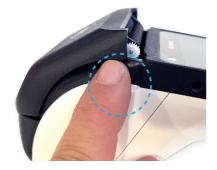
Open paper roll cover of the T650c as shown above. There are small slots to aid opening if required 2
