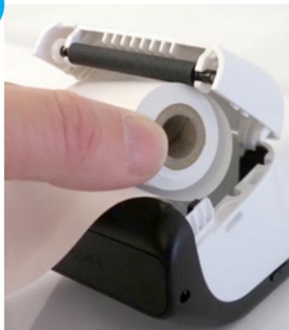
Remove used paper roll. Insert new roll so the paper feeds from the top, leaving a length of paper sticking out of the terminal
